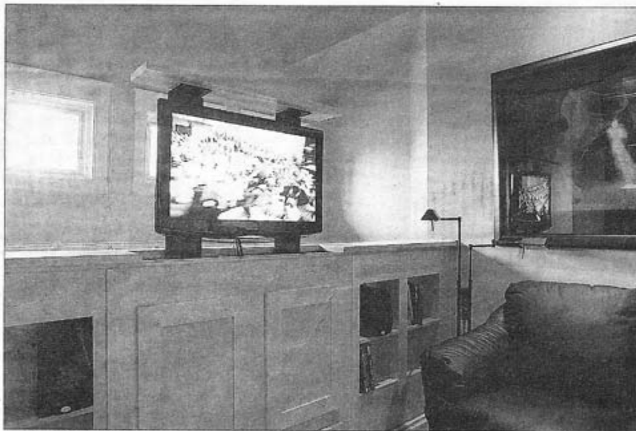
A push of a button exposes or conceals this sitting-room TV attached to a power lift.
